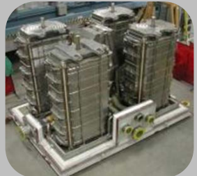
Four-Stack Module 1.4 megawatts
